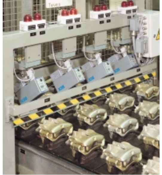
▼ LUT 1-4 luminescence scanners used to ensure that brake callipers for vehicles are correctly fed in.
