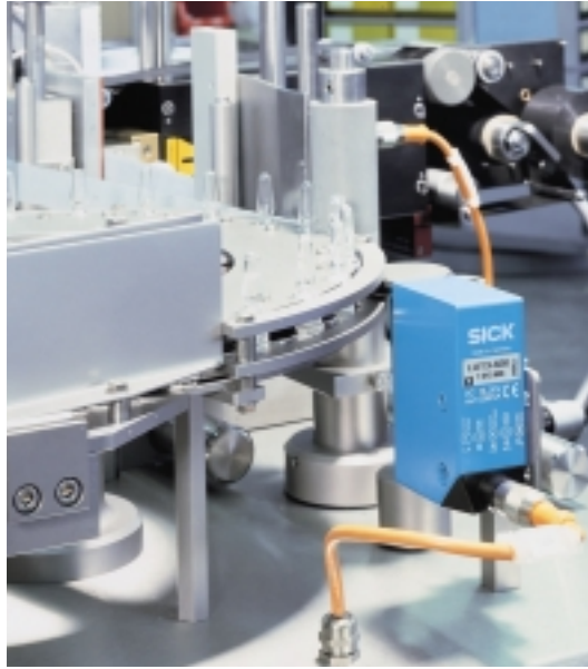
◀ Label present or not: the LUT 3-8 knows the answer (here being used in the pharmaceutical industry).
