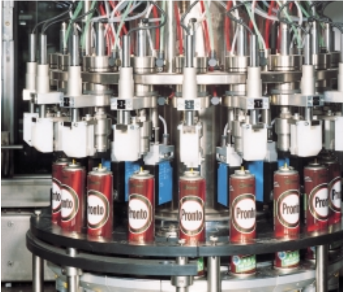
▲ Luminescence scanners being used to align aerosol cans.
